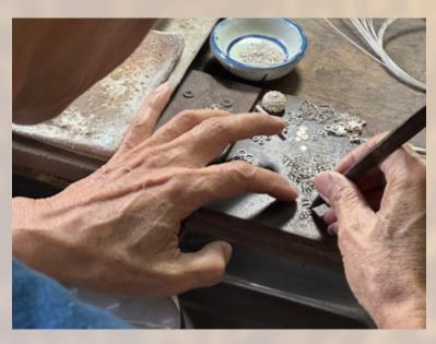
The main components of the inlay work are the structural wire, the inner wire or inlay wire, and the solder.
